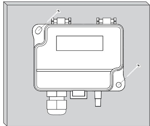
**Figure 1b - Mounting orientation**
