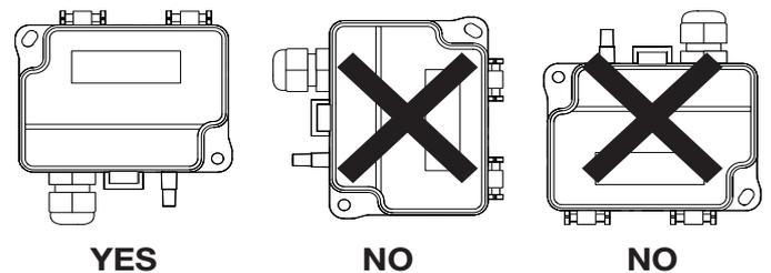
**Figure 1c - Application connections**
