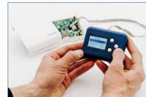
AVEC LE SIRO-CT, IL EST POSSIBLE DE METTRE EN SERVICE DES APPAREILS SIRO SANS ÉCRAN
