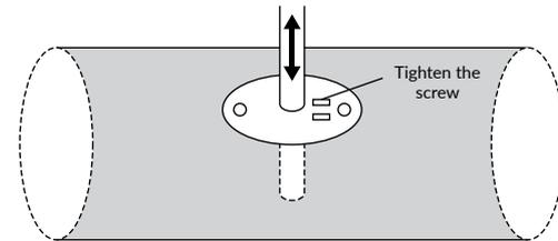
Figure 1c - Mounting orientation
