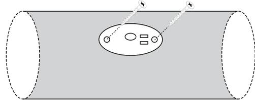
Figure 1b - Mounting the probe in a flange
