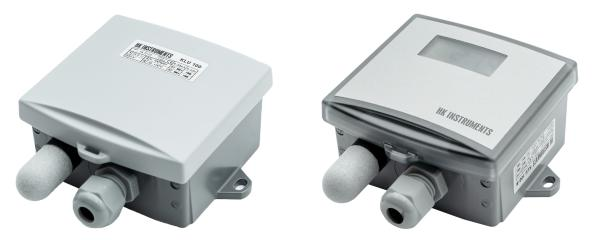
KLU 100 temperature and humidity transmitters are designed for outdoor applications. The transmitter has a capacitive sensor that detects relative air humidity and an NTC10 sensor for temperature measurement. A sintered plastic filter protects the sensor elements.
